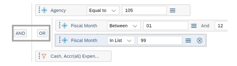
In this example, we have added another set of objects to the query filters. We can use drag and drop to create another nested query filter for the second set of program/subprogram filters.
